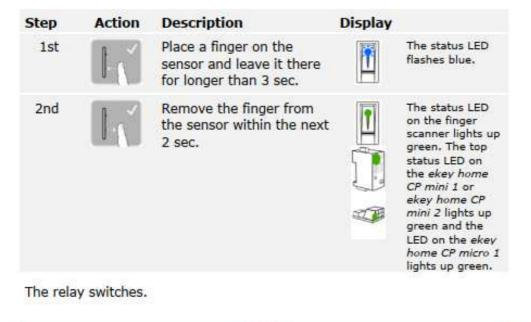
This means that you can keep your finger on the sensor for up to 5 sec. If the finger is kept on the sensor for longer than this, the relay will not switch.
